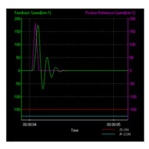
Figure 7: Untuned system (Purple plot: Reference velocity, Green plot: feedback velocity)
