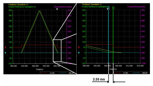
Figure 10: Settling time less than 4 msec with Yaskawa Sigma-5 servo
