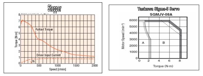
Figure 2: Comparison of torque speed curves between a stepper and a servo of comparable size.
