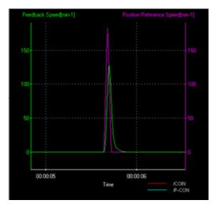
Figure 8: Tuning-less function enabled (Purple plot: Reference velocity, Green plot: feedback velocity)
