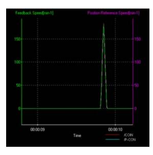
Figure 9: Autotuned system response (Purple plot: Reference velocity, Green plot: feedback velocity)
