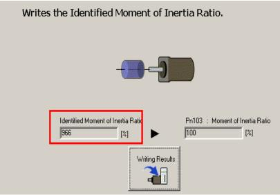
Figure 4: Inertia estimation results
